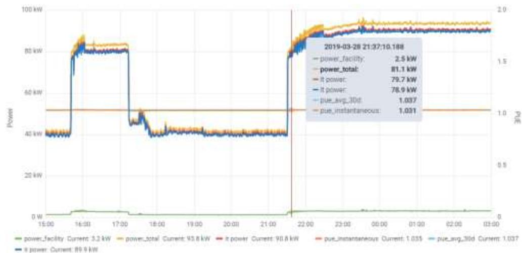
This cooling setup has enabled POD1 of the BodenTypeDC project to run with a thirty-day rolling average PUE of 1.03 meaning that for each kWh of energy consumed by the IT systems, 30Wh is consumed by the facility, namely the cooling fans, power distribution losses and the lights.
